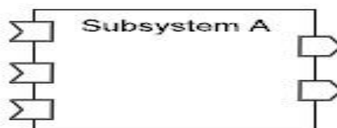
Figure 4. External view of a subsystem with three input message ports and two output message ports.
